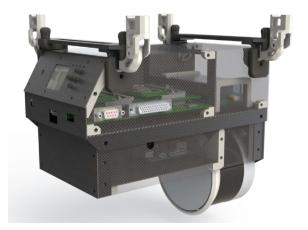
The payload controller with the LiDAR payload.
