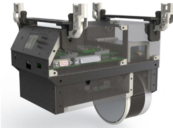
*The payload controller with the LiDAR payload.*
