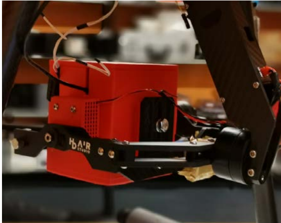
Thermal payload mounted on gimbal
