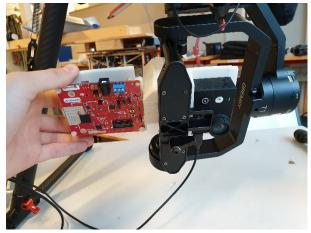
The surface water velocity drone payload
