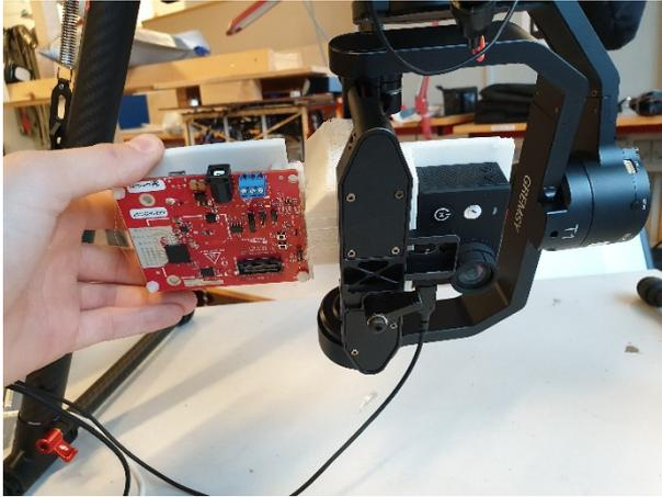
*The surface water velocity drone payload*
